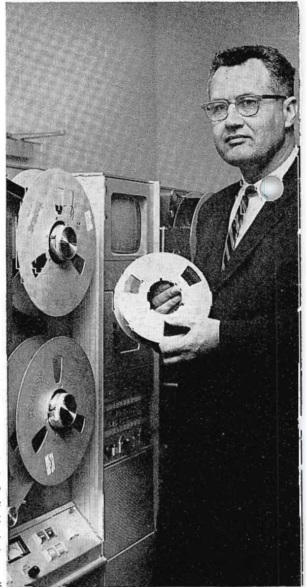
SPECIAL 8-INCH TAPE REEL used to conserve space, save on reel and shipping costs. This accommodates the usual half hour program. Mr. B. W. Spiller, station manager, uncovered a source for the cost-saving product.
